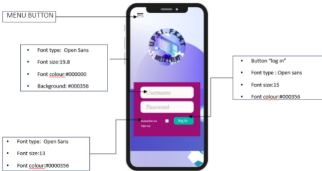
Diagram 3.2: Description for screen Log in main menu for META Student and Admin
