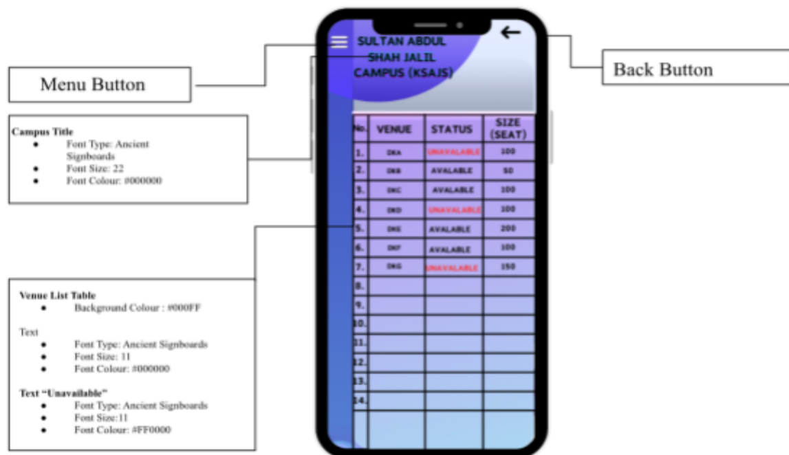
Diagram 3.31: Description for screen which show the venue information in KSAJS for META Student and Admin
